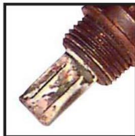
Ethylene Glycol (Antifreeze) Contamination
